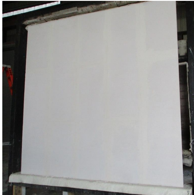
Photo No. 3 Exposed face of Wall Assembly – (Pre-Test)
