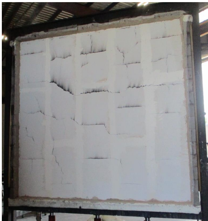
Photo No. 8 Exposed Face – (Post-Fire Resistance Period)
