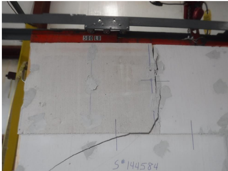
Photo No. 16 Example 1 of Racking Test Failure (Wood Frame)
