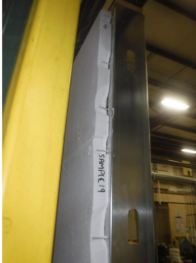
Photo No. 15 Example 3 of Racking Test Failure (Steel Frame)
