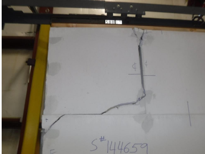
Photo No. 13 Example 1 of Racking Test Failure (Steel Frame)
