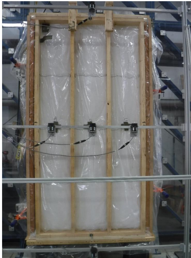
Photo No. 4 Uniform Static Load Test Setup (Wood Frame/Negative Pressure Direction)
